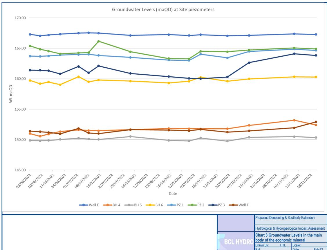
2.8.3.7 Prior to the quarry development (and the associated dewatering operation), it is postulated that the groundwater flow direction would have been from south southwest (peaking at 164-167 maOD in the vicinity of PZ1, PZ2, PZ3 & Well E); and declining towards the north northeast (equating to 158-160 maOD at BH6).
