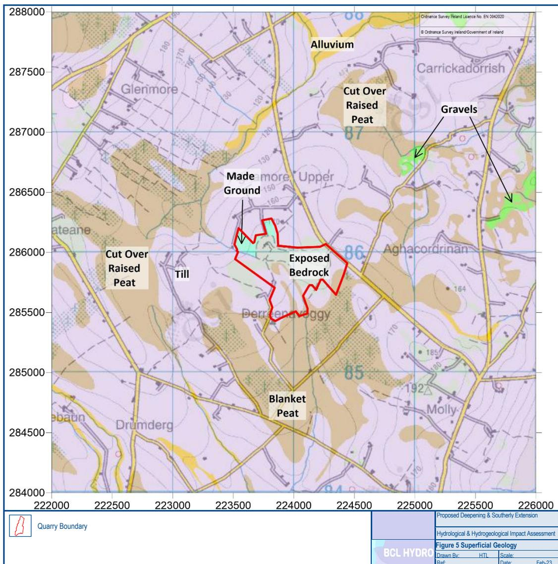
2.5.3.2 Beyond the exposed bedrock in the quarry void and the made ground (stockpiles) in the northwest part of the landholding, the surrounding lands have an extensive cover of Till (derived from Lower Palaeozoic sandstones and shales).
