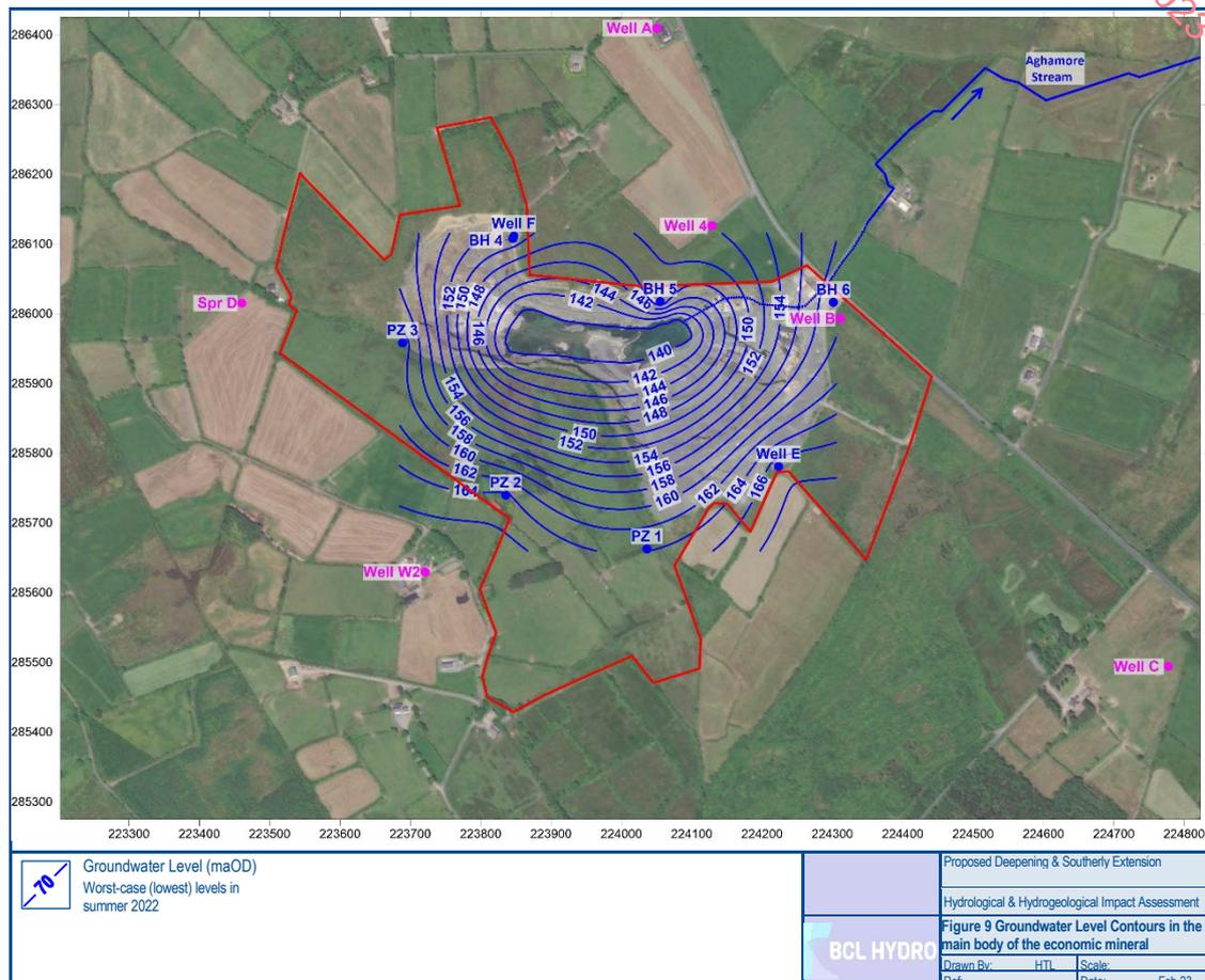
2.8.3.9 Piezometers PZ1, BH6 and Well E are situated some 200-250 m from the deepest sinking and have been installed at original ground level. Groundwater level at these locations is 2-5 m bgl, demonstrating that they have not been impacted by the dewatering operation.
